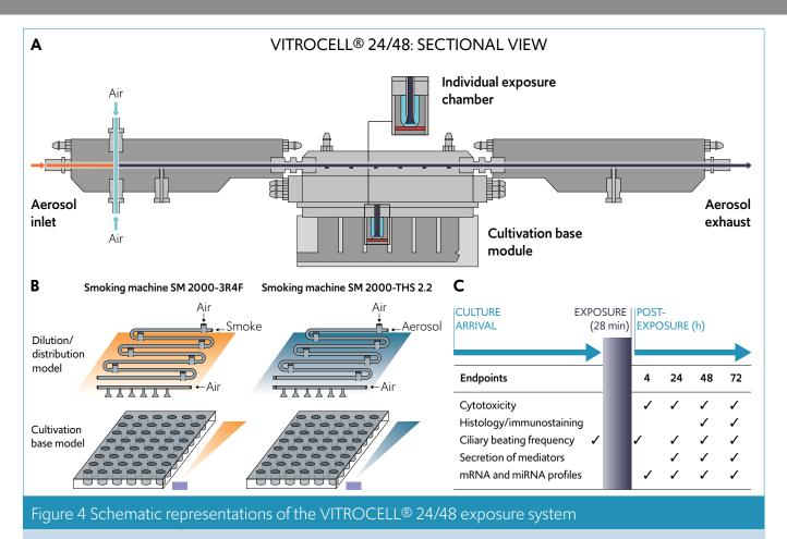
(A) Schematic cross-sectional view of one row showing the dilution/distribution module, the cultivation base module, and individual exposure chambers; (B) Experimental setup for a comparative study of THS 2.2 aerosol and cigarettes smoke; (C) Experimental design of an exposure study of organotypic cell cultures.
